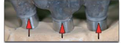
Twisted metal frame due to degassing (with previous model)
